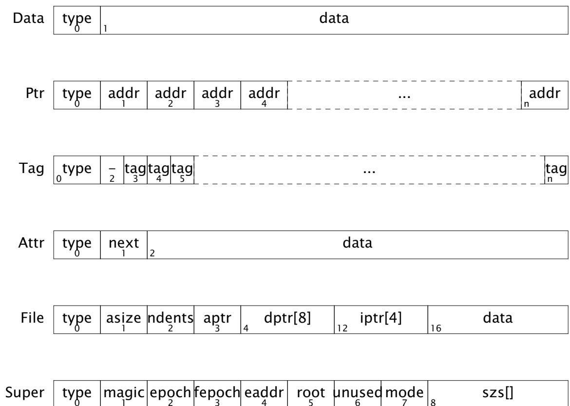
Figure 2 Block types. Numbers indicate the word number (64-bit words). Blocks are usually 16 Kbytes. All disk addresses are 64-bit words, but tags are 32bit epochs. All integer values stored on disk are kept in little-endian format. All strings known by the file server program are kept encoded in UTF-8, including the final Nul byte.
